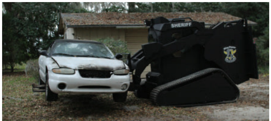
The Rook's vehicle extraction tool can be used to push or pull a parked vehicle or even pick up a vehicle and remove it.
