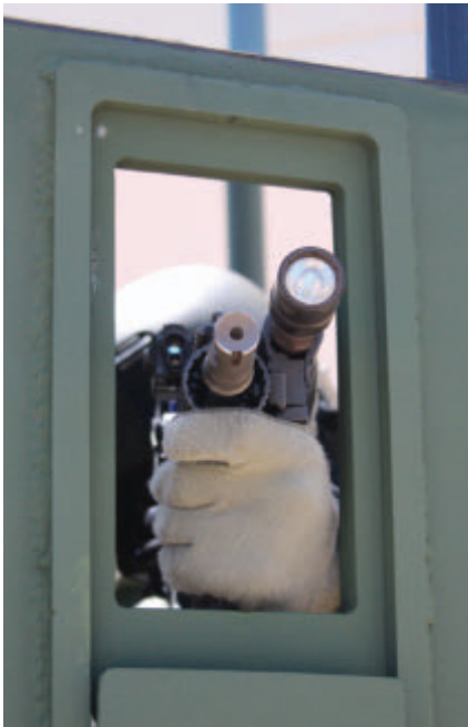
The Rook's armored deployment platform includes two 5 in. x 9 in. sliding gun ports, four bulletproof glass sight ports and video cameras attached to the front of the platform.
