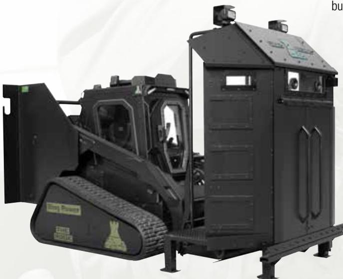
When the Armored Deployment Platform is mounted on the vehicle, the operator can raise it to 11 feet so that entry can be made on both the first and second floors, and the roofs. The platform height is also ideal for airplane assault incidents. In a vehicle take down, the platform can be slanted downward for crowd control and rescues.
