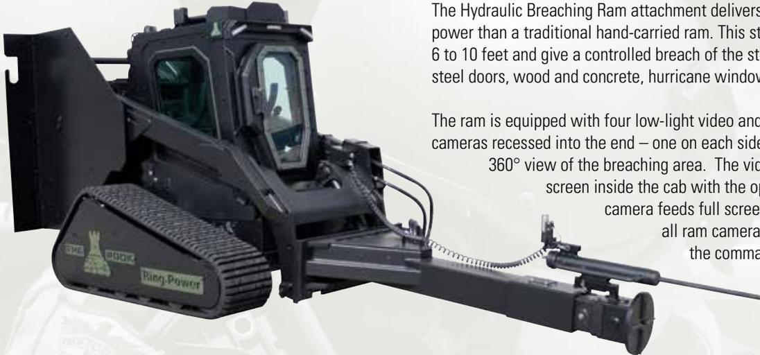
The Hydraulic Breaching Ram attachment delivers 6,500 psi of pressure and much more power than a traditional hand-carried ram. This standard attachment can extend out from 6 to 10 feet and give a controlled breach of the structure including block walls, reinforced steel doors, wood and concrete, hurricane windows and windows protected by burglar bars.
