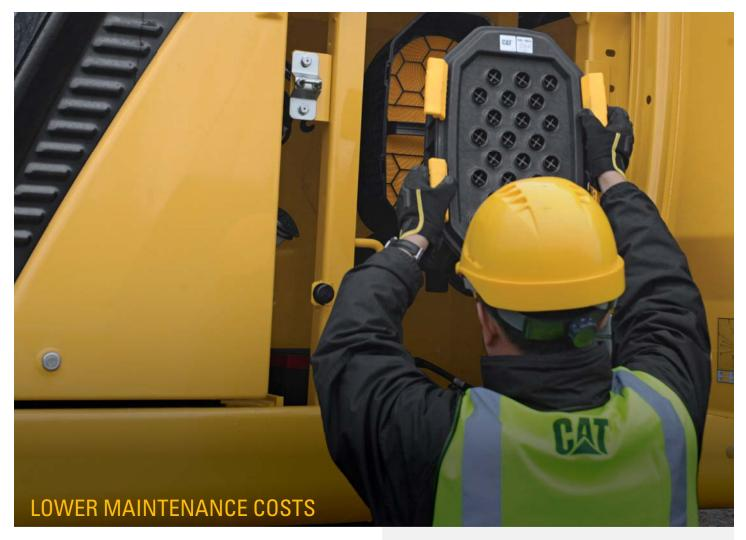
With extended maintenance intervals, you get more done at a lower cost compared to the 336F. Consolidated filter locations make service faster. Hydraulic, air, and fuel tank filters have increased capacity and longer life.
