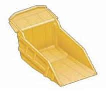
Gateless Coal Body. This specialized high volume body, available in several sizes, is targeted at dedicated coal haulage applications with minimal impact. It eliminates the tailgate with a kicked up floor design that gives the volume required to meet target payload.
