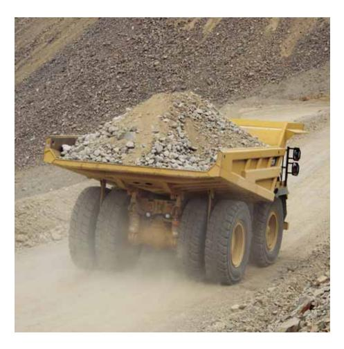
Integrated Braking System. The Cat oil-cooled braking system delivers reliable performance and control in the most extreme haul-road conditions. The integrated system combines the service, secondary, parking brake and retarding functions in the same system for optimum braking efficiency.
